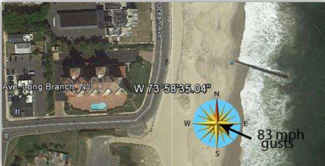
Figure 3: Super Storm Sandy Maximum Wind Speed and Direction at Subject Building
